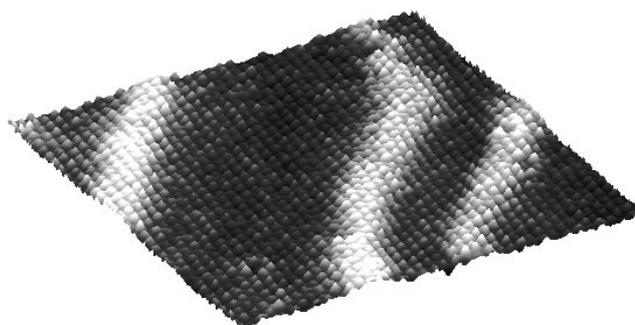
**Fig. 3.** Pseudo 3D image of the Au(111) surface with atomic resolution at 5 K ( $V_t = 0.07\text{ V}$ ,  $I_t = 3.74\text{ nA}$ , scan area  $10\text{ nm} \times 10\text{ nm}$ ). The stripes reflect the  $23 \times \sqrt{3}$  surface reconstruction. This figure represents the topographic raw data with a background correction and a smoothing of four-next-neighbor pixels
