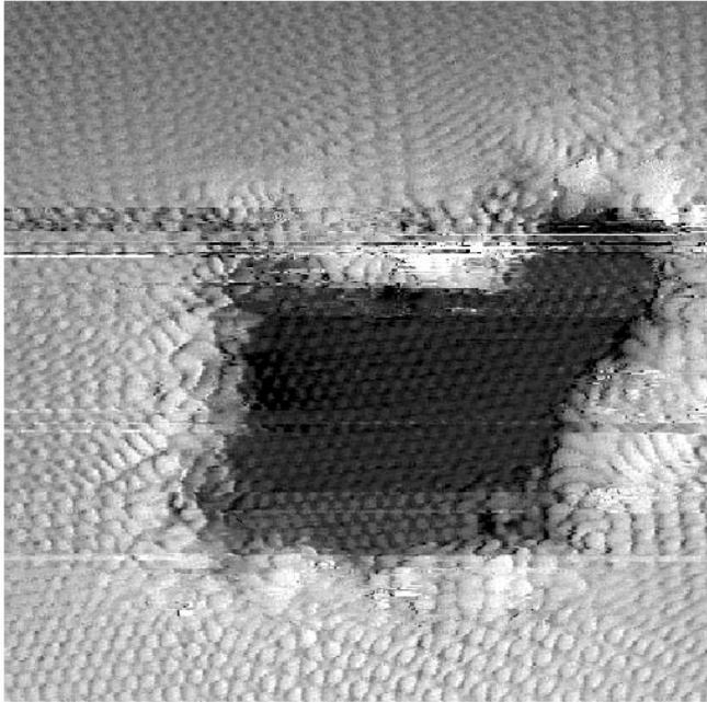
**Fig. 5.** A typical nanopit produced in the HOPG surface imaged at 5 K. Note the atomic resolution also at the bottom of the pit. Parameters:  $V_t = 0.10$  V,  $I_t = 0.69$  nA, scan area  $10.4$  nm  $\times$   $10.4$  nm. The STM data were differentiated to enhance the grey-scale contrast on the atomic level
