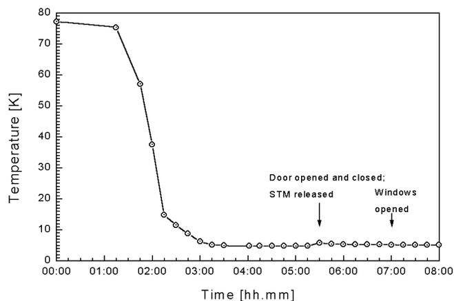
**Fig. 2.** Temperature measured near the position of the sample as a function of time during cooling down from 77 K (LN<sub>2</sub> temperature) to 5 K. Note the slight increase in  $T$  when the door is opened for several minutes. No temperature rise is observed, however, when opening the infrared-shielded windows
