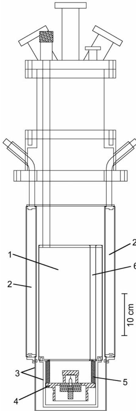
**Fig. 1.** Schematic of the cryogenic set-up of the LT STM with the STM body hanging in its concentric copper housings at the bottom of the cryostat: (1) LHe dewar, (2) LN<sub>2</sub> dewar, (3) concentric copper cylinders with doors and windows, (4) STM block, (5) three springs, and (6) tubes for springs. Not shown are the door mechanisms and the stainless steel wires to firmly pull up the STM body and press it against the bottom of the LHe dewar for cooling down or tip and sample exchange
