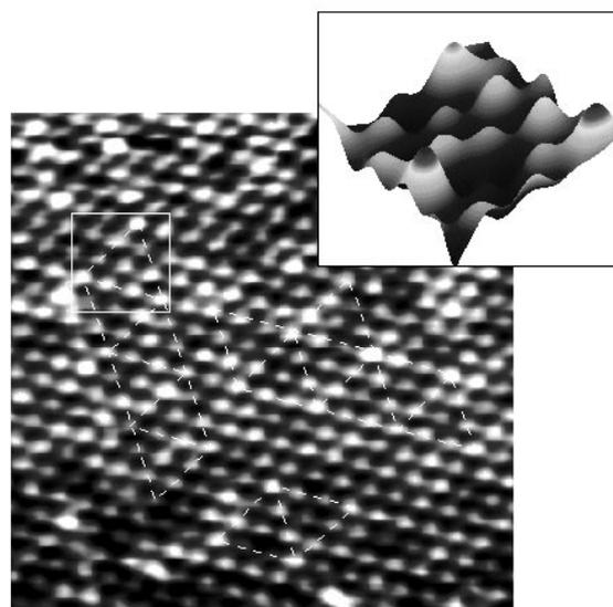
**Fig. 4.** Top view image of the NbSe<sub>2</sub>(111) at 5 K surface with atomic resolution. Clearly visible are the three domains of the charge-density wave (dashed lines). A pseudo-3D image of the square section is shown as an inset. Parameters:  $V_t = 0.02\text{ V}$ ,  $I_t = 2.55\text{ nA}$ , scan area  $5\text{ nm} \times 5\text{ nm}$ . The STM data for this figure were low-pass filtered in the Fourier transformation
